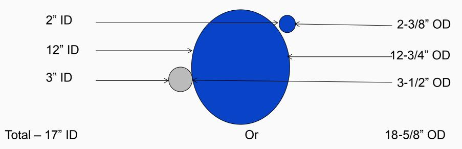
What is the correct minimum borehole size?
