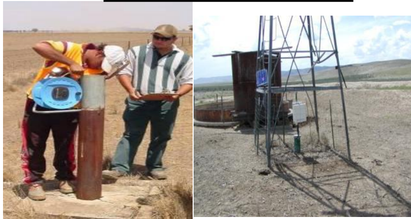
Manual/Automatic Groundwater Monitoring
